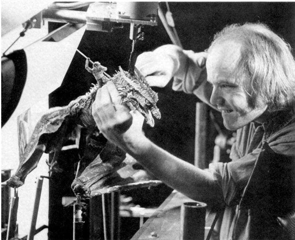
Phil Tippett makes an adjustment to the go-motion controlled dragon armature from Dragonslayer .
